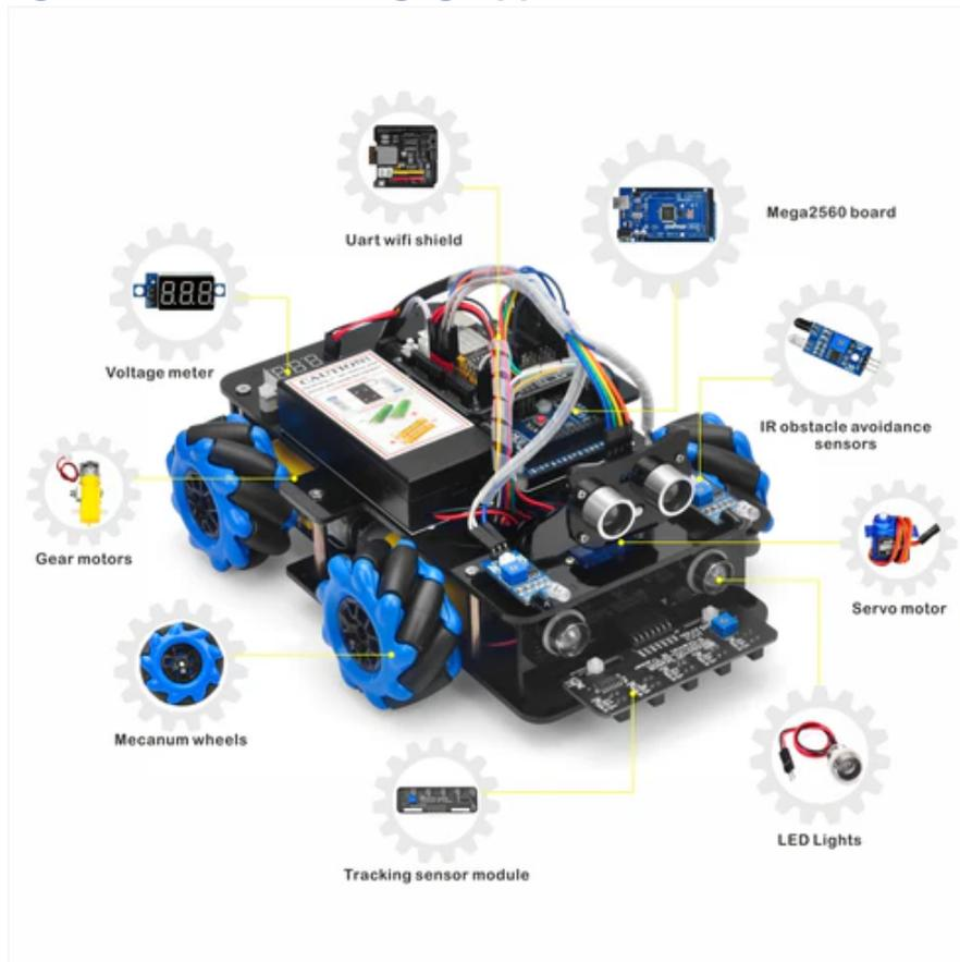
Abbildung 4: V2 Mecanum Wheel robot car
